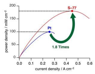
Figure 4. Power density *versus* current density produced from fuel cells with platinum and  $H_2$  as S-77 as the anode catalyst and platinum as the cathode catalyst.
