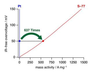
Figure 2. iR–free overvoltage *versus* mass activity. (At an iR–free overvoltage of 50 mV, platinum: 0.859 A mg<sup>-1</sup>, H<sub>2</sub>ase S–77: 547 A mg<sup>-1</sup>)
