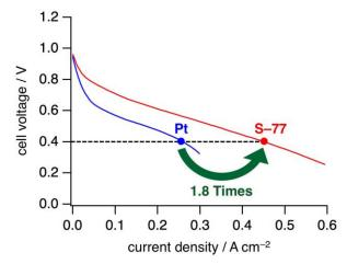
Figure 3. Cell voltage *versus* current density produced from fuel cells with platinum and  $H_{2}$  as S-77 as the anode catalyst and platinum as the cathode catalyst.
